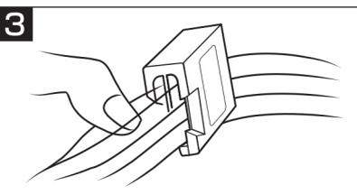
When the rails are partway inserted, with the divider between them, press down diagonally and continue pressing downwards.
