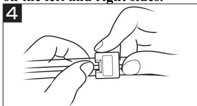
Once the slider has clamped down on the rails, push it downwards, until it snaps into place.
