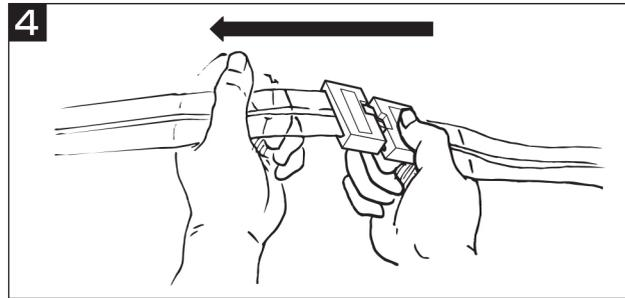
Move the sliders together. Once the sliders have docked, move them left and right a few inches to completely seal the bag. Should reopening the bag become necessary, open as in step 2.
